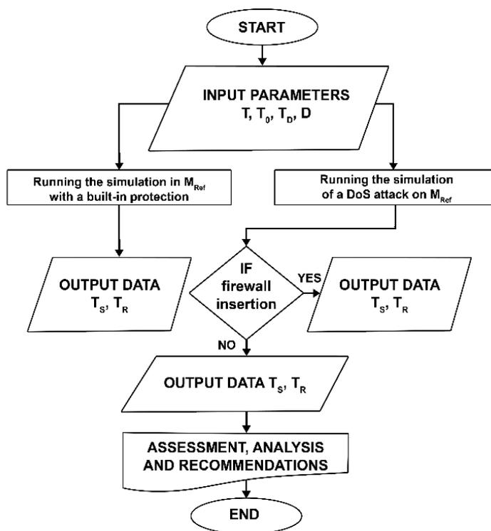
Fig. 4. Algorithm of simulating a DoS attack on a management center.
